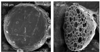
Fig. 1. Photomicrograph of casein microparticles coacervated with protamine. The upper numbers indicate the total width of the picture.
