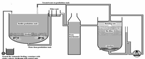
Fig.1. Schematic view of the recirculation system.
