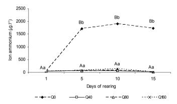
Fig. 1. Means values of ammonium ion levels (μg.l<sup>-1</sup>) during the *L. alexandri* rearing with four different biofilter media quantities (0, 40, 80, and 160g.l<sup>-1</sup>). Different capital letters showed significantly difference (P<0.05) between different biofilter media quantities in the different days of samples. Different small letters showed significantly difference (P<0.05) inside of each treatment during the time.
