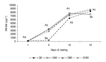
Fig. 2. Means values of nitrate levels (µg.l<sup>-1</sup>) during the *L. alexandri* rearing with four different biofilter media quantities (0, 40, 80, and 160g.l<sup>-1</sup>). Different capital letters showed significantly difference (P<0.05) between different biofilter media quantities in the different days of samples. Different small letters showed significantly difference (P<0.05) inside of each treatment during the time.
