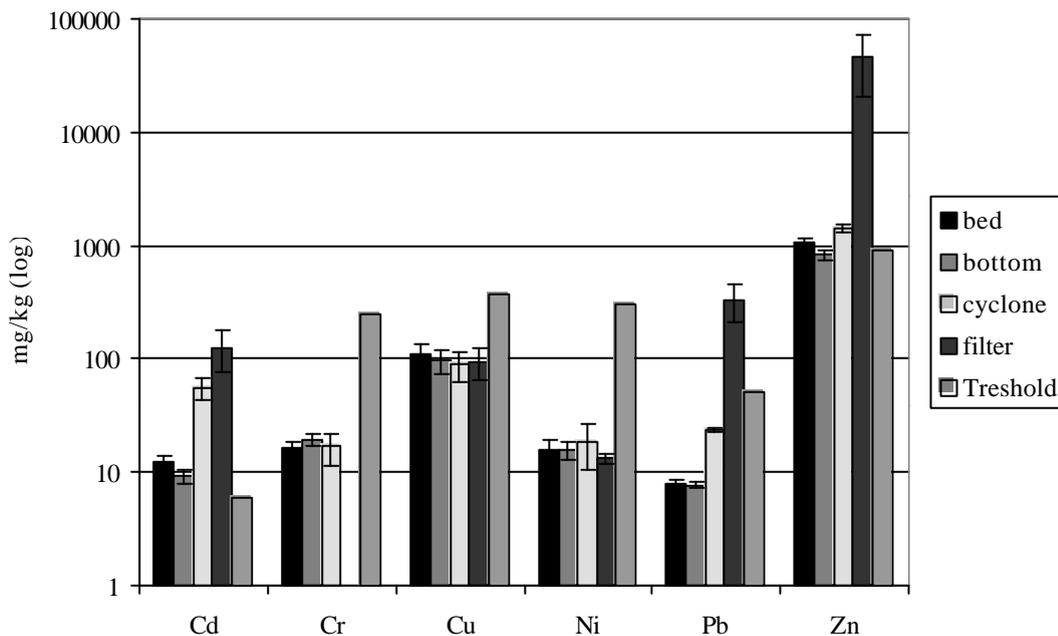
Figure 6–4: Average metal concentrations (mg/kg) of different ash fractions compared to the VLAREA threshold concentrations for fertilizer.
