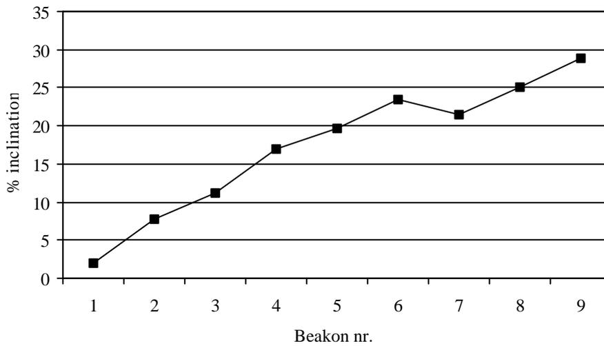
Figure 7-11: Percentage inclinations compared to the original sediment thickness for each of the beacons in October 2000
