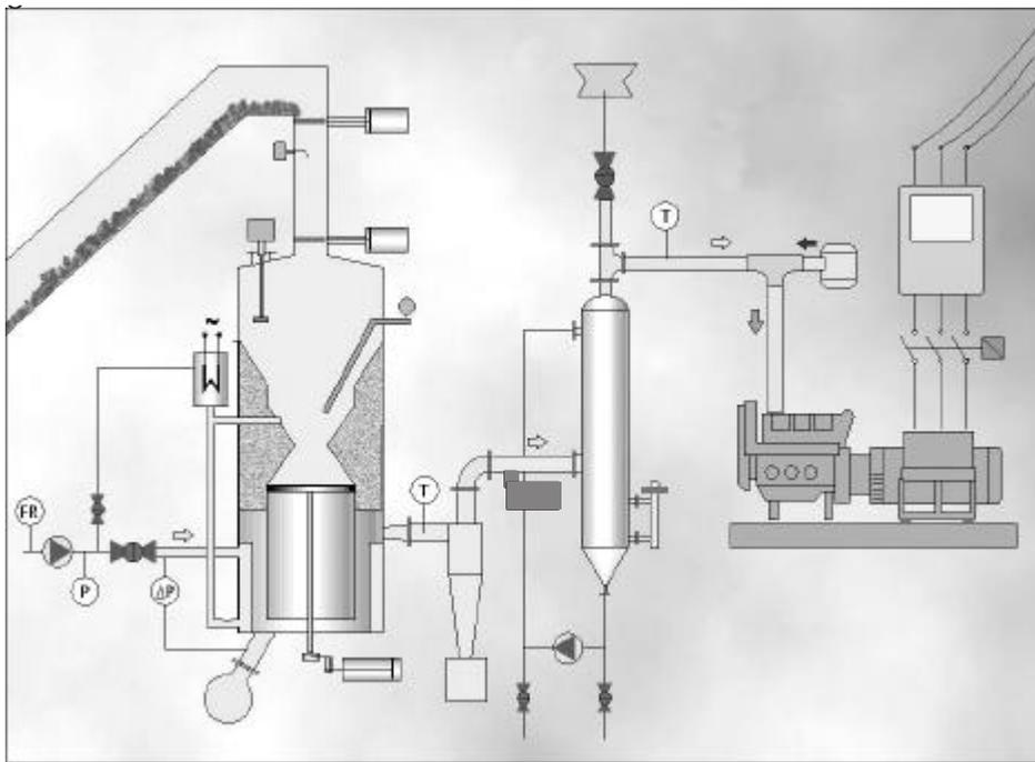
Figure 6–1: Scheme of the fixed bed downdraft gasifier used in the tests with the locations of sampling the different ash fractions: 1) gasifier boiler, 2) gasifier bed ashes, 3) bottom ashes, 4) cyclone ashes, 5) filter fly ash sampled in condensation unit, 6) scrubber, 7) cogeneration unit.
