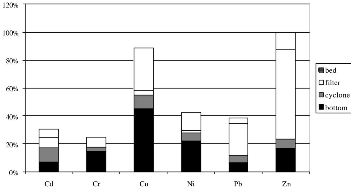
Figure 6-3: Heavy metal material balance (100%: metal input from willow wood)
