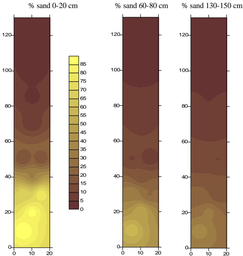
Figure 7-5: Sand content (%) at 3 depths (0-20 cm, 60-80 cm, and 130-150 cm) of the new sediment layer
