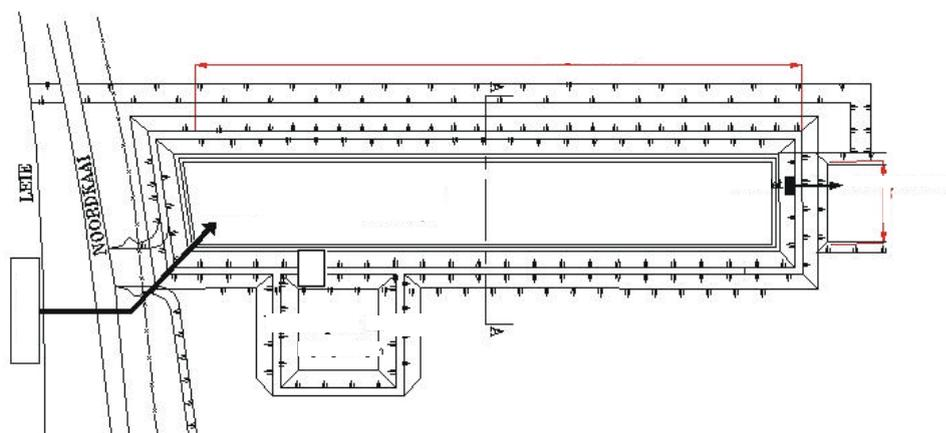
Figure 7-2: Diagram of disposal sites A and B with their new embankment.
