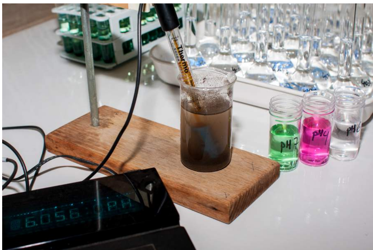
Measurement of soil acidity with an electrode after shaking dry soil in demineralized water or KCl solution
