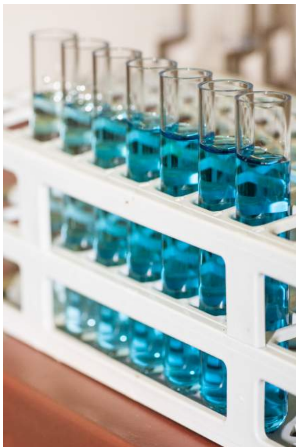
Colorimetric determination of phosphorus in extractions from biomass or soil samples
