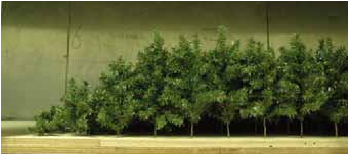
Fig. 4.2: The gradual transition consisted of three rows of model trees with increasing height towards the edge of the model forest. In this photograph, the crown depth of the model trees of the stand itself was 0.24 m and the trees were set in a stem density of 100 \text{ ha}^{-1} .
