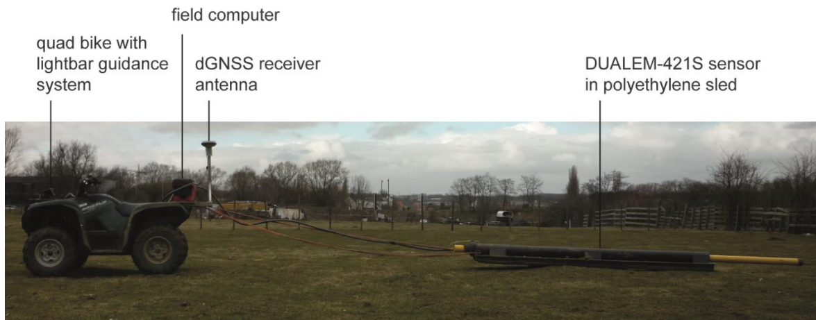
Figure 3.6 Mobile EMI survey configuration illustrated for the DUALEM-421S sensor; the photograph was taken at the landfill site discussed in case study IV in Chapter 5, more specifically in survey zone 5.
