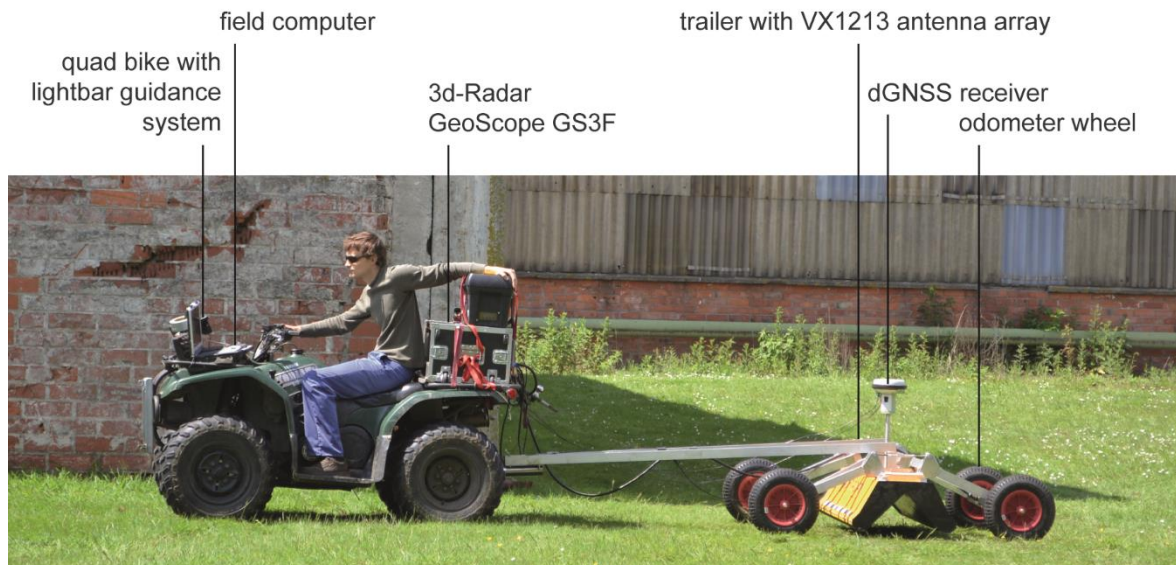
Figure 3.10 Mobile survey configuration of the 3d-Radar GeoScope GS3F SFCW system in combination with a VX1213 antenna array; the photograph was taken at the industrial site discussed in Chapter 7.
