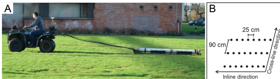
Figure 7.2 Mobile EMI survey configuration with the DUALEM-21S sensor mounted in a sledge behind a quad bike (A) and a schematic representation of the sampling pattern (the illustration here includes three parallel survey lines) (B).
