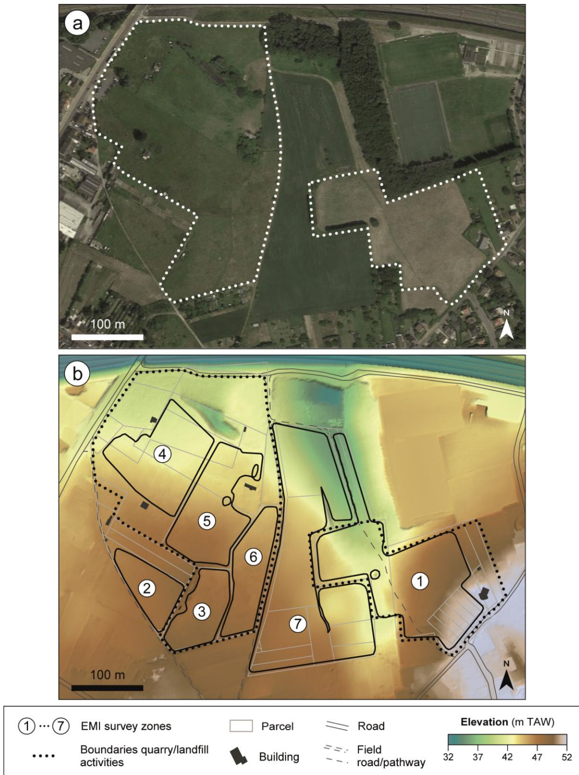
Figure 5.11 (a) Satellite image of the study area considered in landfill case IV (source: Google Maps, Imagery ©2015, Aerodata International Surveys, Cnes/Spot Image, DigitalGlobe) and (b) local DTM with the elevation expressed in m TAW (AGIV, 2014), overlaid by the cadastral parcel boundaries, buildings, roads included in the LRD (AGIV, 2016b), and digitized field roads and pathways. The seven separate survey zones are outlined by black contours.
