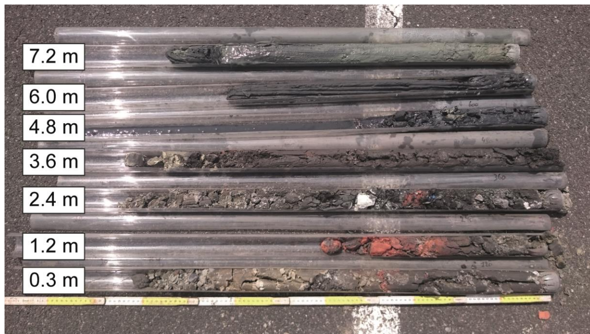
Figure 5.9 Soil cores collected at drilling location 4 down to a maximum depth of 8 m. The labels indicate the start depth of the different liners.
