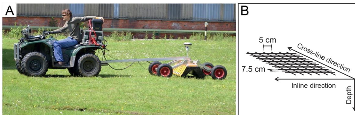
Figure 7.3 Mobile GPR survey configuration with the V1213 antenna array mounted on a trailer pulled by a quad bike (A) and a schematic representation of the horizontal sampling pattern within a single scan track (B).
