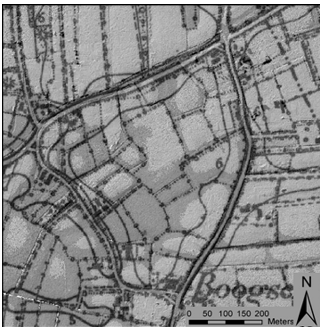
Fig. 6. Overlay of a historical map of 1909 (Military Cartographic Institute) with the enhanced TIN visualized as a hill shade elevation model. Elevation varies from 5.2 to 7.0 m.
