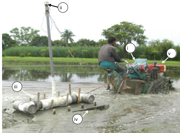
Fig. 1 The floating soil sensing system (FloSSy) during field measurement of EC_a . The different components are indicated as follows: i laptop, ii GPS, iii water proof sensor housing, iv floating platform, v the power tiller
