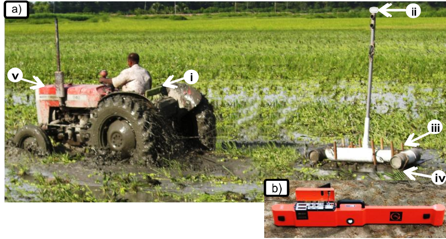
Figure 9.1. (a) FloSSy with: (i) laptop (protected by a plastic sheet), (ii) GPS antenna, (iii) waterproof sensor housing with an EM38-MK2 inside, (iv) floating platform and (v) power tiller; (b) EM38-MK2.
