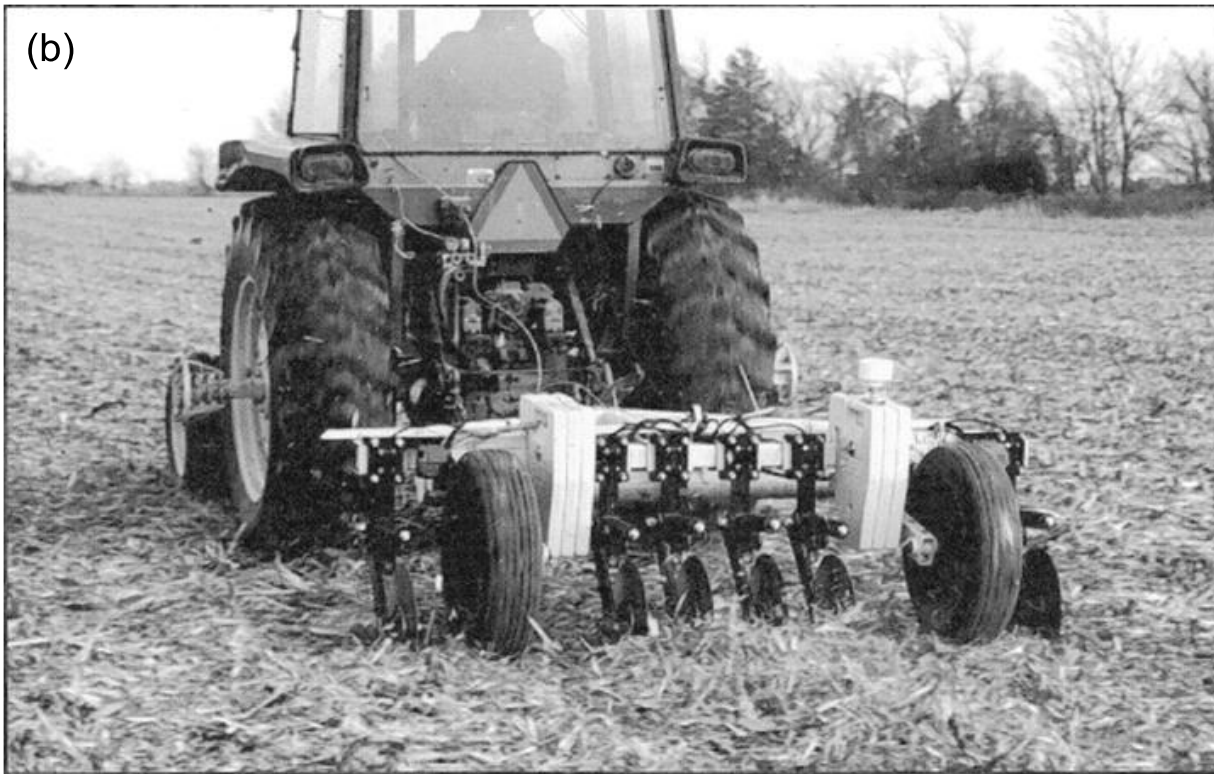
Figure 2.1 (a) Basic principles of galvanic electrical resistivity measurements and (b) illustration of a mobile ER survey equipment: the Veris 3100 system.
