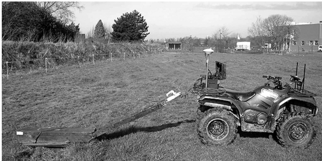
Figure 2.2 Illustration of a mobile EMI survey equipment.
