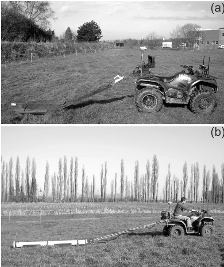
Figure 3.3 Sensor platforms of the EM38-sensors (a) and the DUALEM-21S sensor (b) in action.
