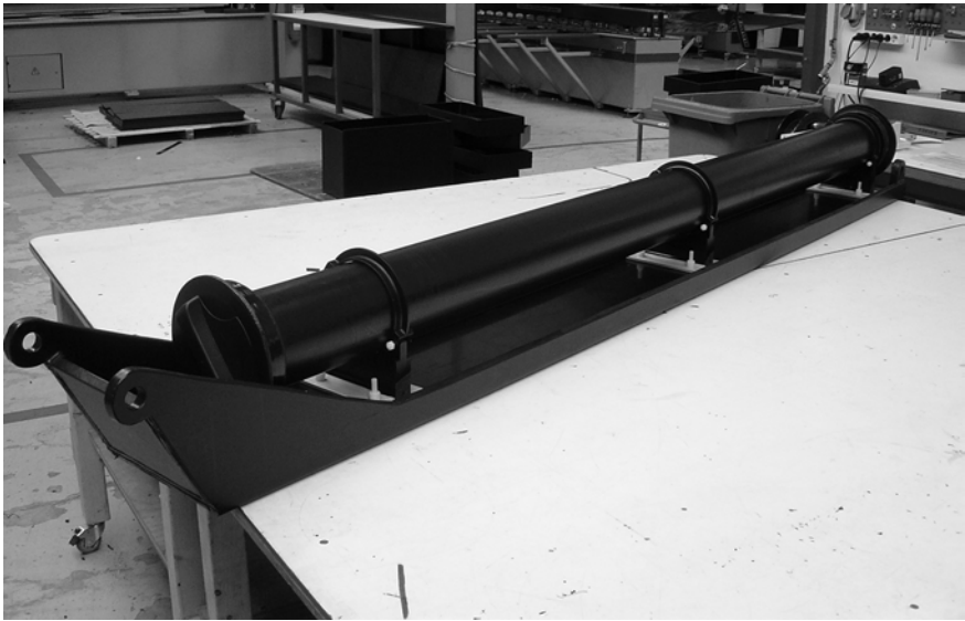
Figure 3.2 Custom-made sled of the DUALEM-21S.
