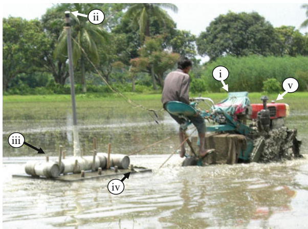
Fig. 1 FloSSy with: (i) laptop (protected by a plastic sheet), (ii) GPS antenna, (iii) waterproof sensor housing with an EM38 inside, (iv) floating platform and (v) power tiller
