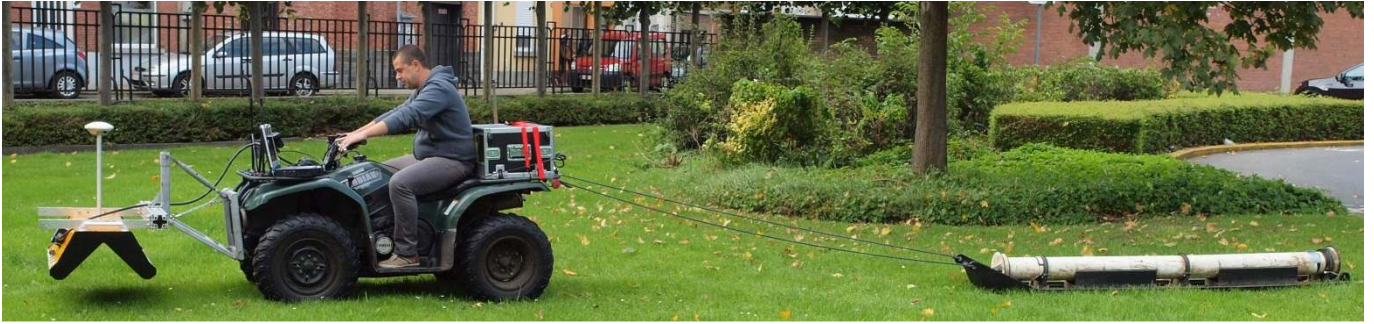
Fig. 3. A mobile GPS-positioned geophysical soil sensing systems with two sensors: in front a suspending ground penetrating radar antenna-array, in the towed sled an electromagnetic sensor.
