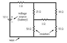
The diagram has a few symbols, such as the symbol for a voltage source (this could be for example a battery). Voltage sources generate a force which causes electric currents to flow in the circuit. The voltage source shown is rated at 10 volts (V). This means that the voltage is 10 volts higher at the + or wide-line side of the battery than at the - or narrow-line side of the battery. As a result, electric charges are given a force in the upward direction (from the - side to the + side).
