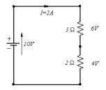
Notice the directions of the voltage arrows across each of the devices. Also notice that the voltage drops across the two resistors are proportional to their resistances. This is called the **Voltage Divider Rule**. This rule is useful in many situations. Suppose that we replaced the above circuit by the one shown here.
