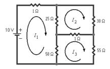
Write down Kirchoff's Voltage Law for each loop. In particular, we see in the left loop that the voltage of the battery is 10V. So, this is the voltage through the resistors of the left loop in total. There are 3 resistors in this left loop. The resistor of  $1\Omega$  is only being influenced by  $I_1$ . The other 2 resistors are being influenced by 2 current loops, in opposite direction through the resistor. So we have to take the
