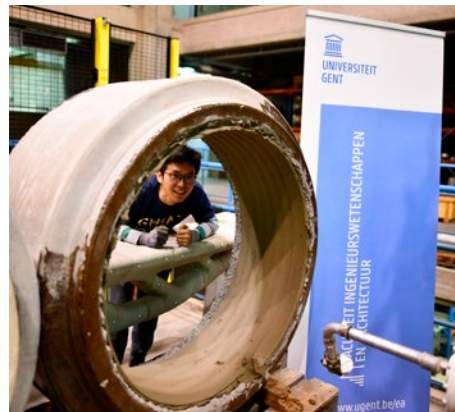
PhD student Tao Yaxin performing experiments on 3D printing of tunnel linings
