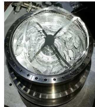
A turbopump at JET with a broken blade due to an unexpected failure.
