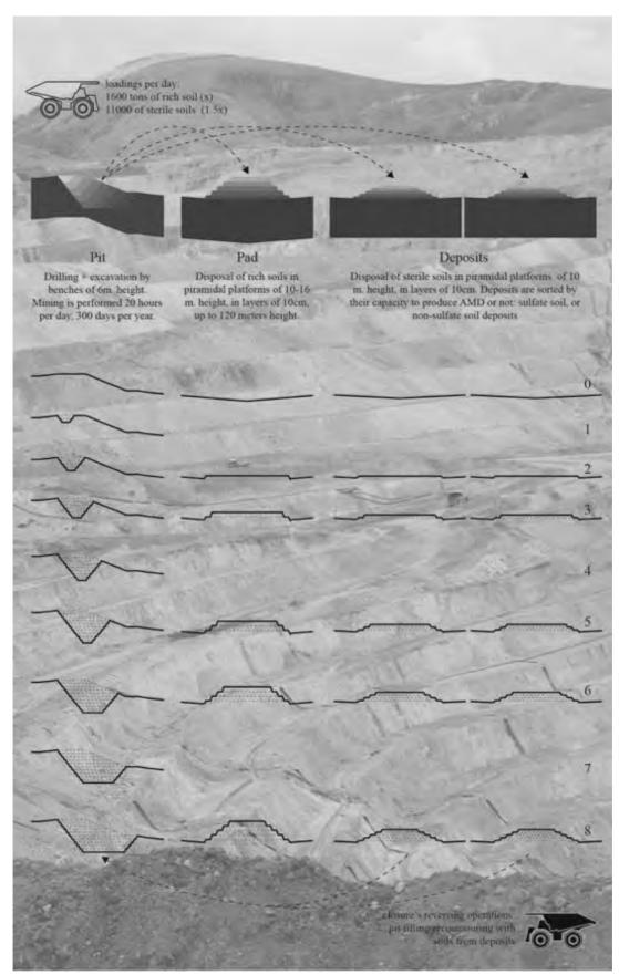
[fig.6] Spatial formation of mining landscapes. Constructive logic of pits, pads and deposits in Yanacocha mine, Cajamarca. Source: elaborated by the author from 'Introduction to Open-Pit Mining' (A. Wetherelt, K. Wielen, 2011) and Yanacocha's Environmental Impact Study (SVS Ingenieros S.A.C., 2010).
