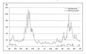
Illustration of water flow in the Kjørbekk creek along the year (l/s), yellow-median value, grey-minimum value. Made by Multiconsult in 2017.
