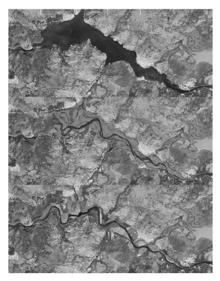
[fig.4] [Hypothesis of] Evolution of Copco lake on Klamath river after the demolition of the Copco No.1 dam. Source: from US Department of Interior, 2012. Elaborated by the author.
