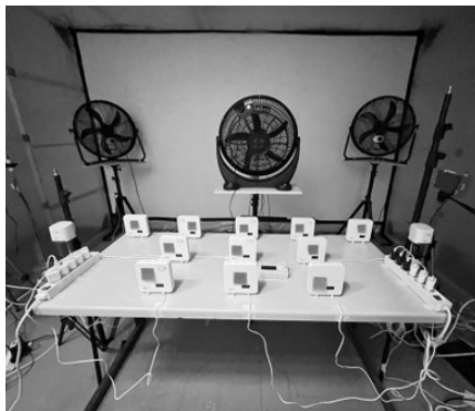
Example of a test set-up for PM sensor calibration
