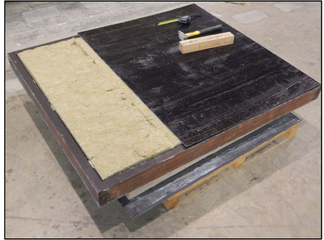
Figure 2. Construction of the dummy window
