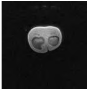
Fig. 3. ZTE image of a pig bone with a resolution of 1 mm and NSA = 16. The image is acquired with the head coil.
