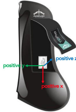
Figure 2.3: Tendon boot with accelerometer [7].
