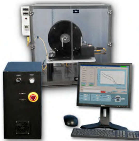
FIGURE 5.6: The RX550/650 (Machine Solutions) designed to measure and record radial reactive force during expansion and compression of interventional devices [182]
