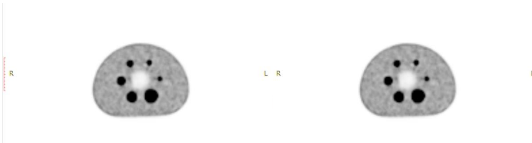
Figure 4-7: Image of PET phantom corrected by the standard CT protocol (left) and the suggested low dose protocol (right)
