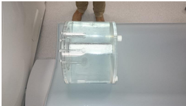
Figure 2-8: PET phantom with fillable spheres
