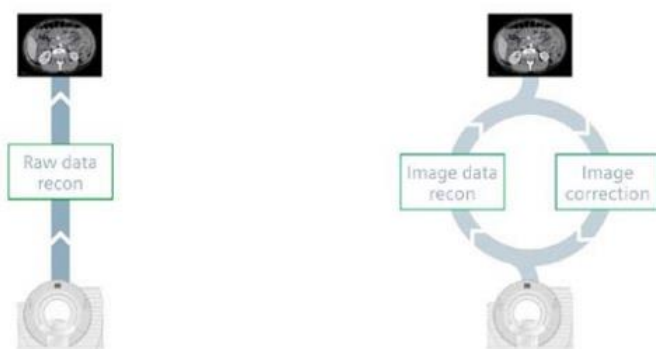
Figure 1-10 Standard filtered backprojection (left) and iterative reconstruction (right) 18
