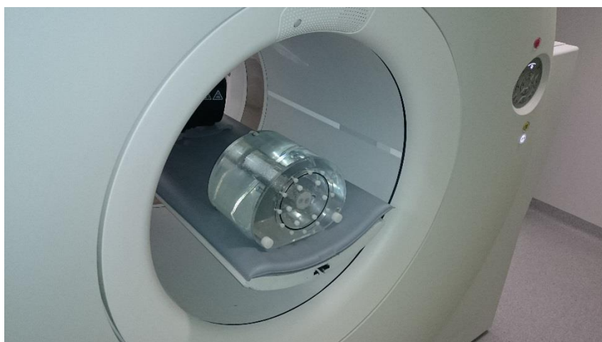
Figure 2-10: PET phantom with activity inside PET-CT scanner
