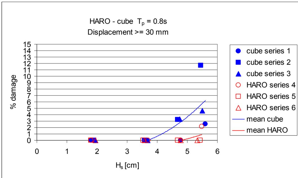
Fig. 3. Damage as a function of the measured significant wave height  $H_s$ .
