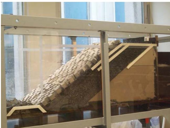
**Fig. 1.** Construction of the model breakwater, armoured with concrete cubes, in the wave flume.
