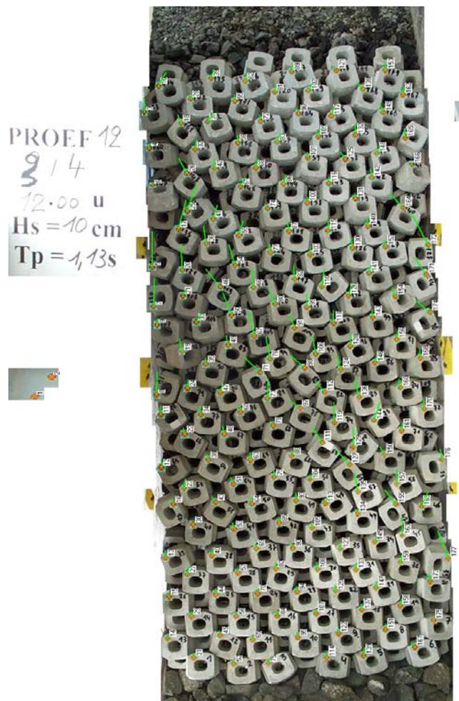
**Fig. 2.** Armour layer of the breakwater: view from above after wave attack. The green lines represent the displacement of the individual HARO units.
