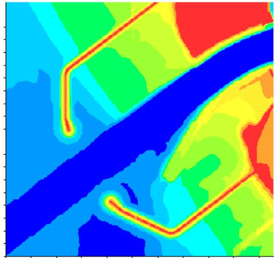
**Fig. 2.** Bathymetry of the planned new design of Oostende Harbour, used for the numerical simulations.
