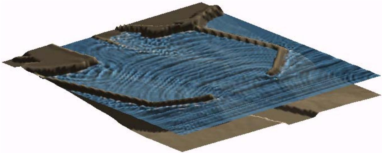
**Fig. 3.** Typical simulation result showing the instantaneous surface elevations of the irregular waves propagating and penetrating the harbour area.
