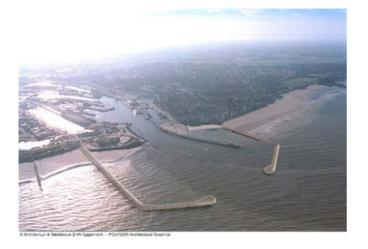
**Fig. 1.** Aerial picture of Oostende harbour with the new port entrance and new breakwaters on the foreground
