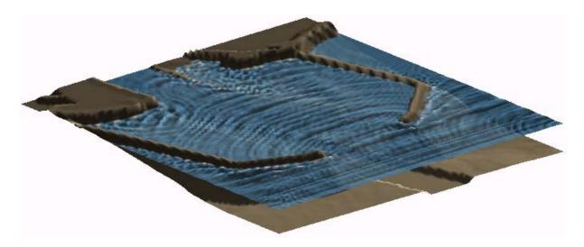
**Fig. 3.** *Typical simulation result showing the instantaneous surface elevations of the irregular waves propagating and penetrating the harbour area.*
