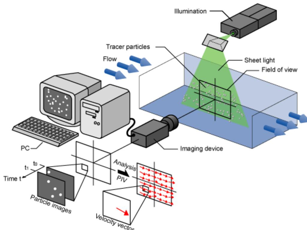
Fig. 1. Principle of PIV measurement.
