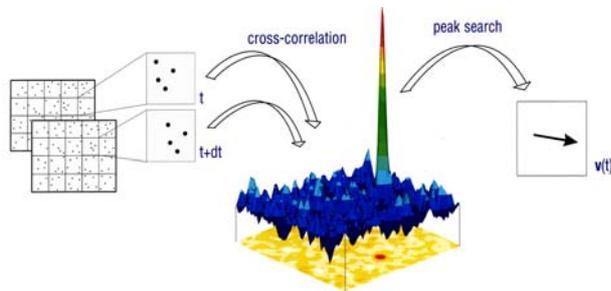
**Fig. 2.** Principle of cross-correlation in PIV
