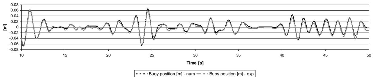
**Figure 3 - Measured and numerically calculated buoy position [m]. Buoy: cone with cylindrical upper part, diameter 31.5 cm, draft = 22 cm, wave characteristics:  $H_s = 6.2$  cm,  $T_p = 1.59$  s.**
