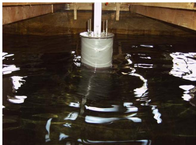
**Figure 2 - Heaving point absorber in wave flume of Flanders Hydraulics Research, Antwerp.**
