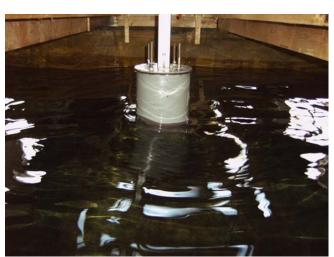
Figure 2 - Heaving point absorber in wave flume of Flanders Hydraulics Research, Antwerp.
