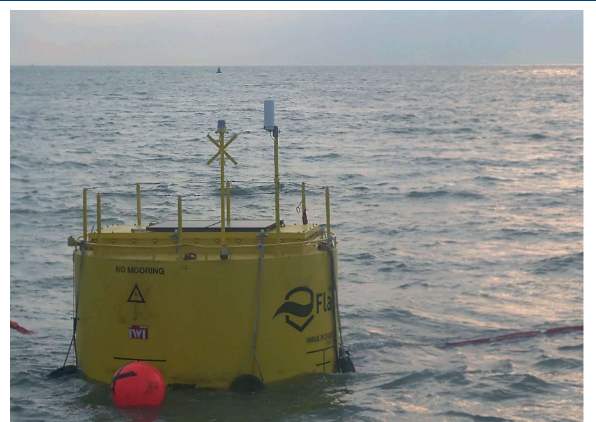
The Wave Pioneer: a prototype (1:2 scale) model of a point-absorber WEC, as a part of the FlanSea project (2007-2010)
