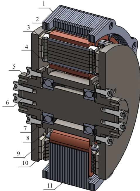
A strong reduction of the core losses is achieved by using grain-oriented material as stator core material. Moreover, the high permeability of these materials reduces the amount of permanent magnet material.
