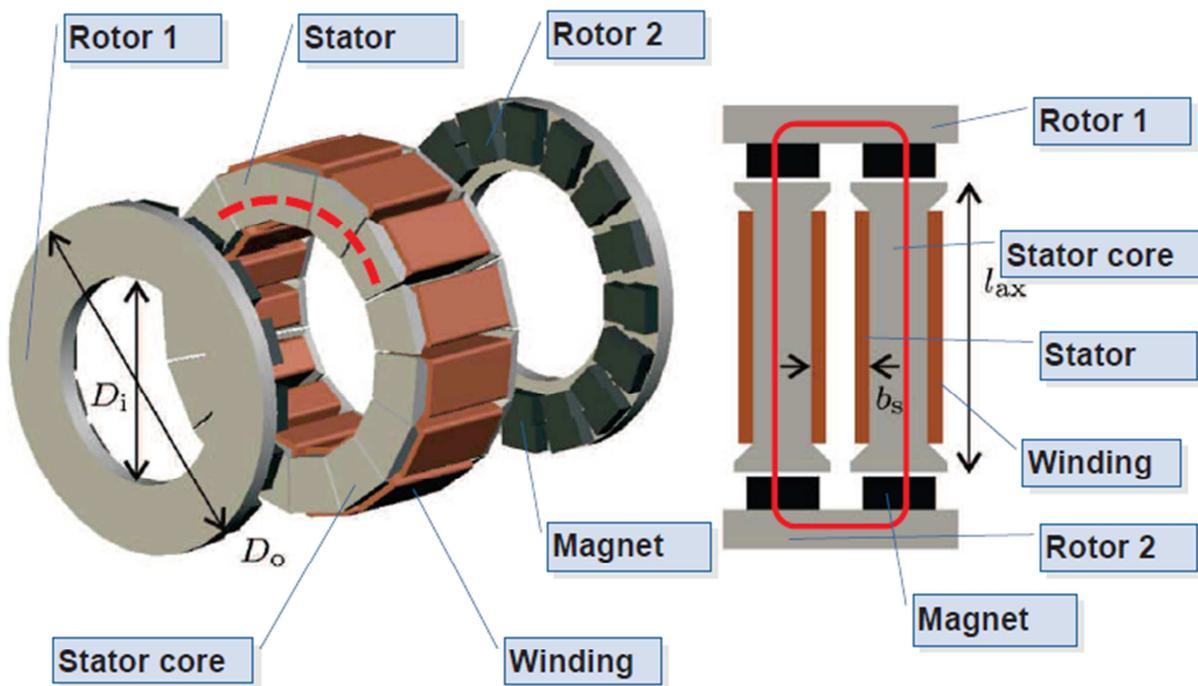
Independent of the topology, axial-flux PM machines inherently combine a high torque density with a good energy-efficiency. Moreover, the high diameter to axial length ratio results in a typical pancake-shape of the machine.
