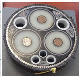
Offshore high voltage cable. Optical fibre is positioned in a white tube.
