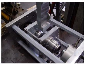
bottom plate of the load-frame. The specimen holders can slide in the horizontal direction to accommodate wear of the friction material specimens. The test box itself is sealed such that it can be filled with a lubricant or with (sea) water to simulate as close as possible the working conditions of the application.
