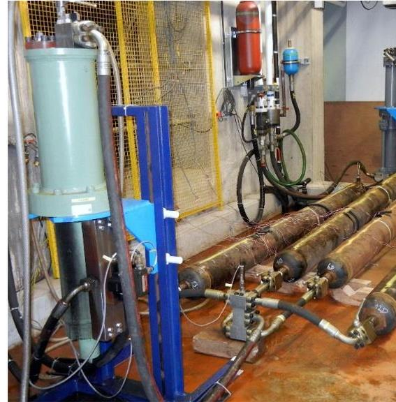
*Figure 1: Simultaneous internal pressure fatigue testing of four 3.5m x 203mm (8") pipe sections between 31bar and 62bar*
