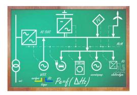
This local grid is made possible by adding a mini-CHP based on an internal combustion engine with hydrogen as fuel and an intelligent control system. The intelligent control, including hydrogen storage and electrical storage, regulates the power balance of the local grid and ensures autonomous behaviour. By autonomous, we mean that the total production can be brought into line with demand at any time on the local grid, without necessarily having to resort to demand control or curtailment.
