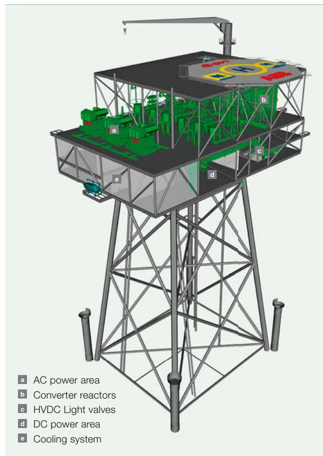
7 An offshore platform for the "Borkum 2" wind farm cluster
