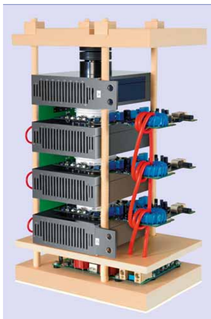
2 Switching unit for the airport radar system
