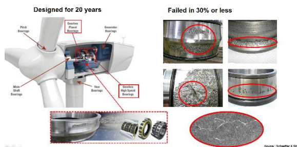
Figure 1 Premature bearing failures in wind turbine gearboxes are associated with White etching cracks [1].
