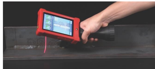
Figure 2: Example of a handheld laser scanner to scan welds.
