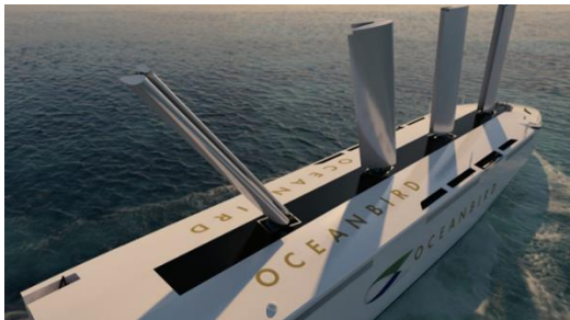
Figure 1: Orcelle - The world's first wind-powered Ro-Ro vessel
