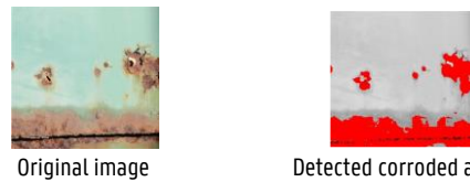
Fig. 4: Image processing technique uses color and texture features in a given image to detect corrosion
