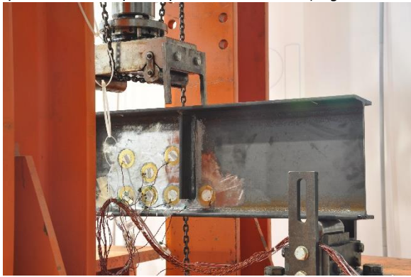
Fig. 3: Medium-scale girder instrumented with piezo transducers.
