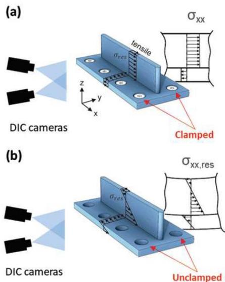
Figure 2: Capturing deformation using DIC through comparing (a): clamped state: unbalanced stress field developed during deposition, (b) unclamped state: distortion leading to redistributed and self-balanced stress field
