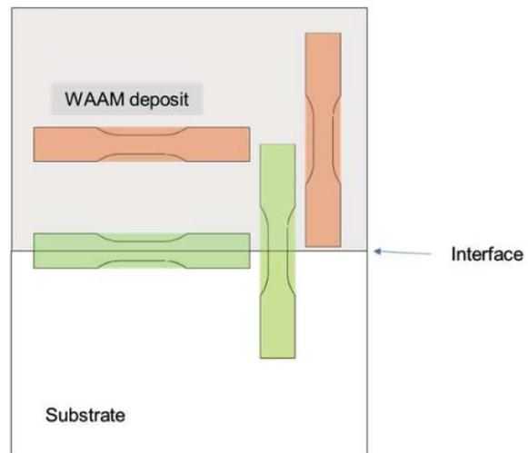
Figure 3: Orientation of dogbone test specimens in the WAAM remanufactured part (green: characterisation of interface; orange: characterisation of deposit)
