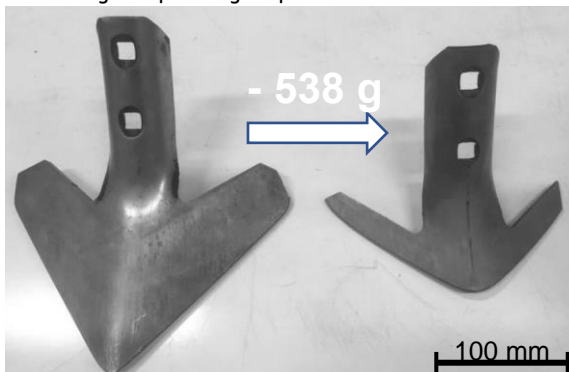
Figure 1 Wear of agricultural tine after 145 km operation in sandy loam
