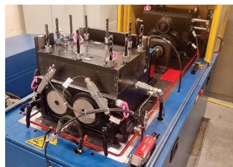
Figure 1: Back-to-back gear tester at Soete Laboratory
