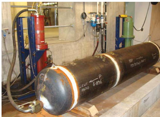
Fig.1. Test vessel ready for fatigue testing under cyclic internal pressure .
