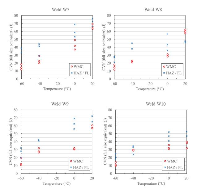
Figure 2: Charpy V-notch transition curves (in terms of impact energy, full size equivalent) of the tested welds.
