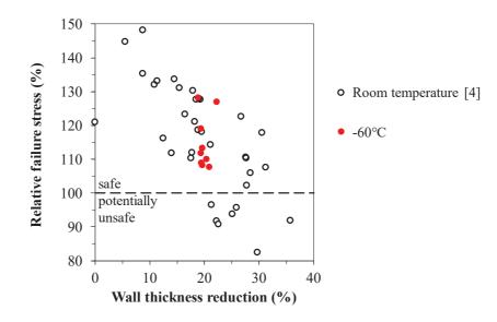
Figure 6: The newly obtained test results at low temperature are located within the scatter band of test results at room temperature.
