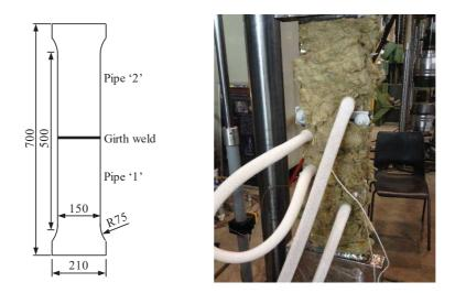
Figure 3: (a) Geometry and nominal dimensions of a Medium Wide Plate specimen. (b) Cooled specimen, insulated by means of Rockwool. White cables indicate the presence of thermocouples to monitor weld temperature during testing.
