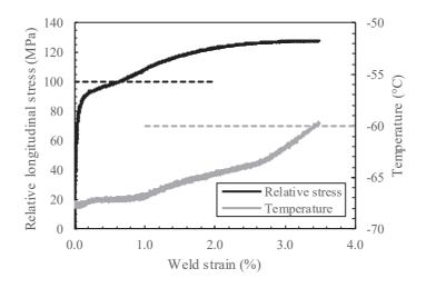
Figure 5: Example test result, depicting relative longitudinal stress and weld temperature as a function of weld strain.
