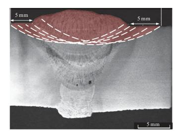
Figure 4: Schematic representation of simulated corrosion damage. Five milling passes are shown; more passes were actually applied to obtain a smooth metal loss profile.
