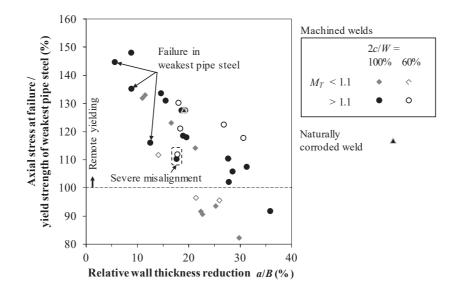
Figure 1: Published results database of load bearing capacity tests performed at Soete Laboratory, Ghent University [4].
