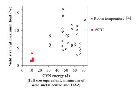
Figure 8: Brittle fracture did not inhibit the occurrence of plasticity within the welds (associated with a weld strain of 0.5%).
