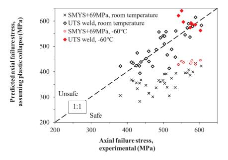
Figure 9: Failure stresses can be accurately predicted by means of a plastic collapse based assessment method (diamond markers), and conservatively predicted when assuming SMYS + 69 MPa as a flow stress (cross markers). The agreement is comparable for tests at room temperature and at -60 °C.
