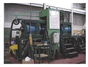
bogies, ... Since self-lubricating bearing materials are often used in offshore technique, the sliding contact zone can be immersed in a water reservoir wherein additions of sand particles or sludge are simulated to provide third body abrasive wear.
