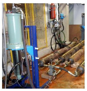
Figure 1: Simultaneous internal pressure fatigue testing of four 3.5m x 203mm (8") pipe sections between 31bar and 62bar
