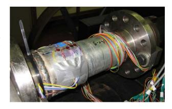
rotates a worm which drives the gear. This causes the male part of the test specimen to rotate with respect to the stationary female part. The resulting torque is transmitted to the lever arm which is connected to the loadcell. The measured load multiplied by the length of the lever arm (1.00 m) equals the acting torque. To allow an axial motion during make-up, a linear guiding system is present.
