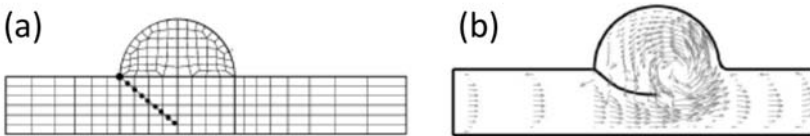
Figure 3.1: (a) Computational domain (b) velocity vectors during the deceleration phase (adapted from [56])
