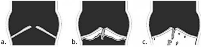
Figure 4.10: Loss of the definition of the VOF in the domain in case of high and reversed \Delta P across the valve. In black the cells filled with fluid, in white the cells filled with void.
