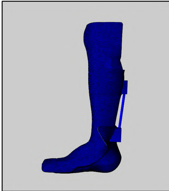
Figure 5.3: Virtual representation of a modular 3D printed AFO together with an entire leg.
