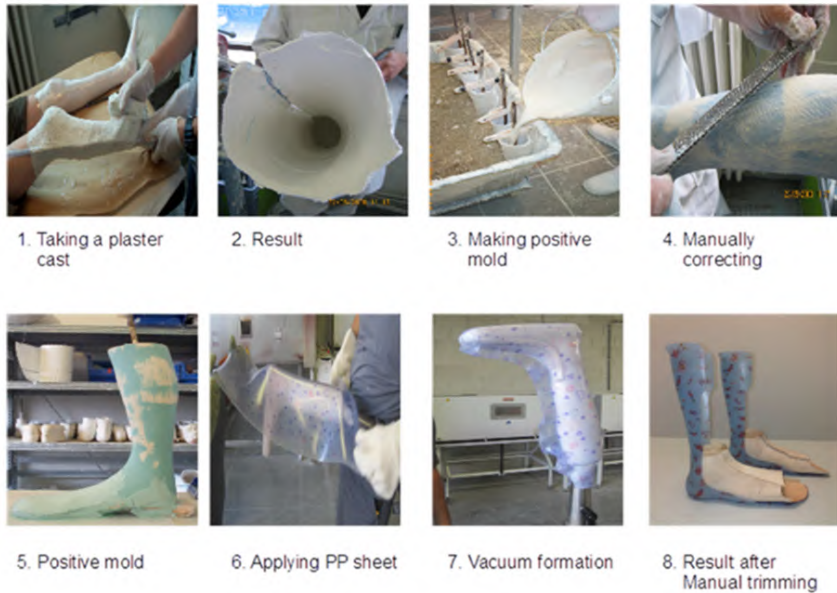
Figure 1.21: Different steps of the manufacturing process for thermoplastic AFOs (adapted from: http://www.sim-flanders.be ).
