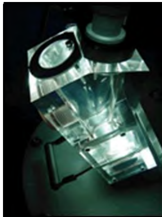
Figure 41: The Dynatek MP4 Robotic Cardiovascular Pulse Duplicator [145].
