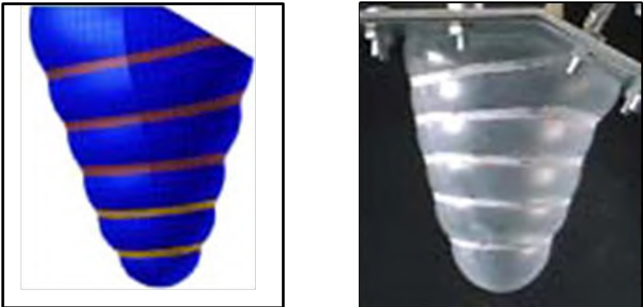
Figure 53: The left ventricular model of Rasponi and colleagues (2006). This figure illustrates the fair agreement between numerical model (left panel) and the ventricle prototype (right panel) at the end diastolic phase. A prominent longitudinal deformation is realized using reinforcement of the silicone wall by circumferential bands. Adapted from [167].
