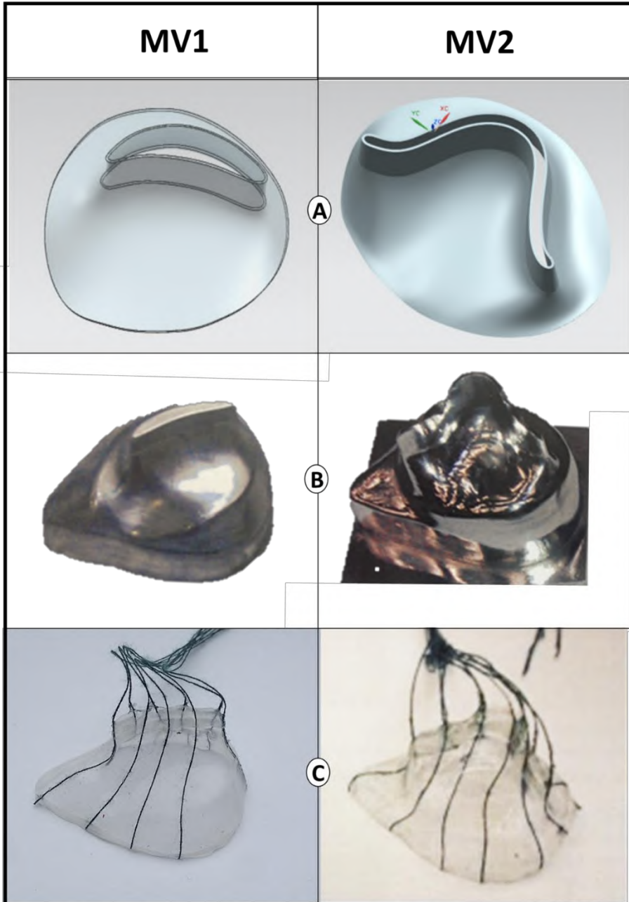
Figure 90: (A) Geometry, (B) aluminum matrix, and (C) in-vitro mitral valve models of mitral valve MV1 (left) and MV2 (right), respectively.
