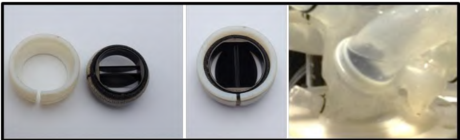
Figure 107: Incorporation of the mechanical bi-leaflet aortic valve into the aorta by a 3D printed valve plane ring (white).
